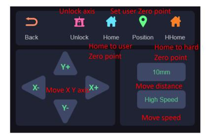
User zero point refers to the position where the user manually confirms that the position of the laser head to the zero. While hard Zero point is the point determined by X and Y limit switch.
