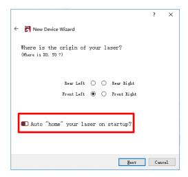
The automatic home function is turned on by default, if you do not want the engraver to automatically home when power on, it is recommended to turn off this function.
