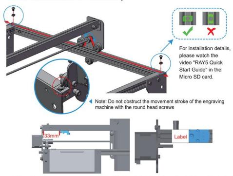
5. Turn the RAY5 engraver over, attach the X limit switch to the edge of the label, and fasten it with a hex key allen wrench, then limit switch is about 33mm from the left sheet metal.
