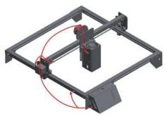
Note: Fix the cable to the sheet metal with cable ties where there is tape, and then move the laser head to the upper right corner to confirm that the cable has sufficient length.
