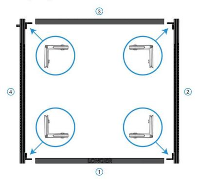
Tighten the M5\*25 screw with M5 washer into frames.
