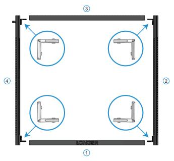
▼ Tighten the M5\*25 screw with M5 washer into frames. Tighten the M5 screws on the corner grooves.
