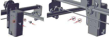
Use a wrench to fix the M3\*6 round head screw, please be careful not to lock the screw, otherwise the laser module cannot be moved up and down.
