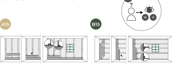
Note: Stagger end joints so they are at least 16" apart. You can usually use the cut end of the previous row to start your new row, but only if the end joints of are at least 16" apart.
