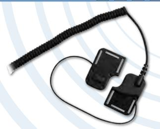
The 5PHK is a bone conduction helmet system specifically design for the Pacific range of  $helmets. Transmission \ and \ receipt \ of \ audio \ is \ via \ the \ users \ skull, this \ enables \ the \ transducers$ to be fully sealed and compatible with many SCBA systems.
