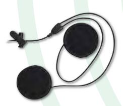
The 5HK is a dual speaker helmet kit. The speaker are enclosed in a low profile cloth housing that includes velcro for helmet mounting. These are a good choice for motorcycle helmets, gliders riot police etc and all helmet applications. This is available with a 2.5mm MONO connector and a 3.5mm screwed connector which is compatible with our 2TACTM throat microphone.
