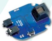
Spare PCB assembly for the model 4SM Speaker Microphone.
