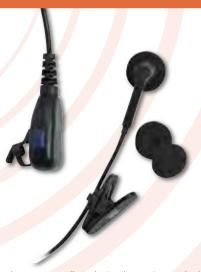
The 2WB is a traditional two wire surveillance kit. It utilizes a 15mm earbud style of speaker. The PTT case includes an integral microphone and rubber PTT button. This accessory is also compatible with our range of Plug & Play accessories. With the addition of the EA-15 Airtube it becomes a cost effective surveillance accessory.
