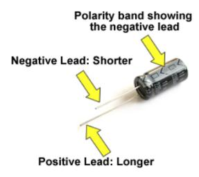
Please pay attention when inserting electrolytic capacitors. Remember to follow the polarity. If the polarity of the electrolytic capacitor is reversed, the capacitor may explode after the power is switched on!!! Always double check all electrolytic capacitors polarity before first power-up!
