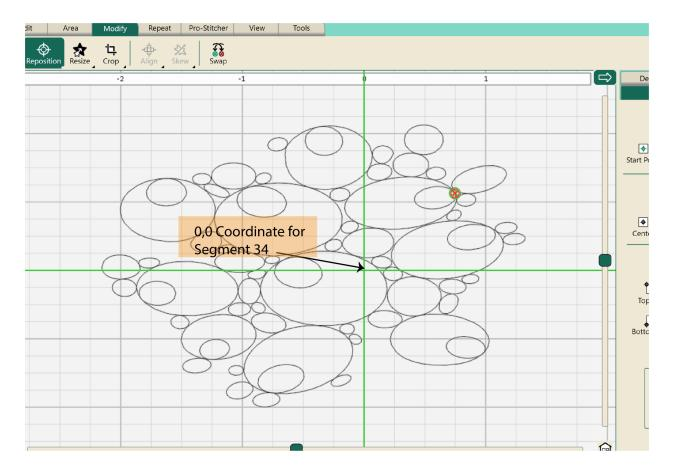
Move your machine to the centre of the panel and then power it on with the Pro-Stitcher This will help line up all the segments
