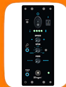
10. BALL LAUNCHER CONTROL PANEL
