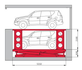
Ensure the bottom of the pit is level, correcting any horizontal errors if necessary. Mark the installation pit based on the actual equipment size. When placing the lifter into the pit, use appropriate steel shims to level it, then fill in the gaps. Additionally, ensure the walls are perfectly vertical.
