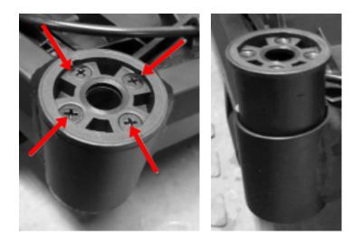
Step 2 : Install new swivel housing by reversing step
