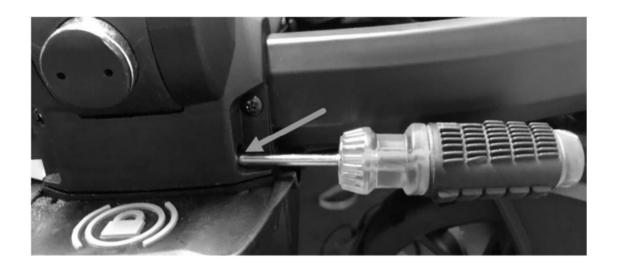
Step 4 : Remove handle pivot covers to expose the handle pivot nut and bolt.
