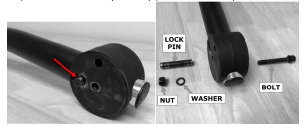
Step 7: Insert the lock pin through the oval port on the new handle. Ensure the lock pin goes through the pull cable port. It is helpful to use a screwdriver to align the pull cable to the lock pin as you insert the lock pin. Verify the handle actuators pull on the lock pin.
