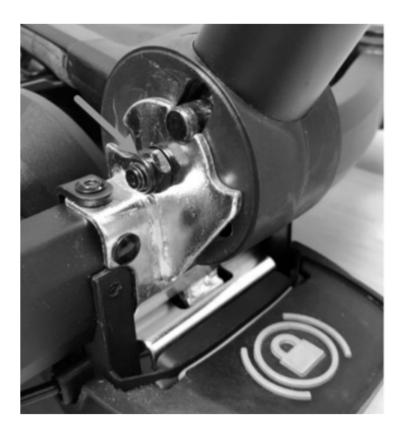
Step 10 : Reinstall the handle pivot covers and screws by following the reverse process of Steps 1, 2, and 3.
