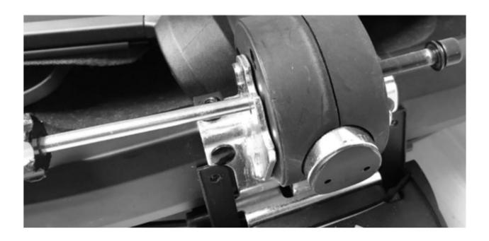
Step 9: Tighten the pivot nut to remove excessive side-to-side handle play. Verify the handle locking pin is able to slide freely to ensure proper handle function. Reference "Handle Locking Pin Function" video for more information.
