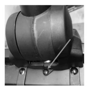
Step 2: Remove two front screws from the Cruiser.
