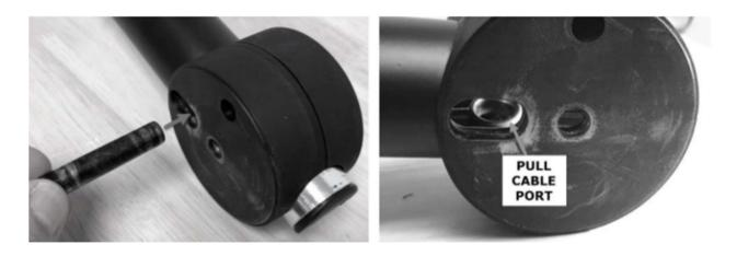
Step 8: Place the new handle onto the cruiser and insert the pivot bolt. To install the pivot bolt it is helpful to use a screwdriver to compress the spring in the lower lock pin as you slide the bolt through the hole.
