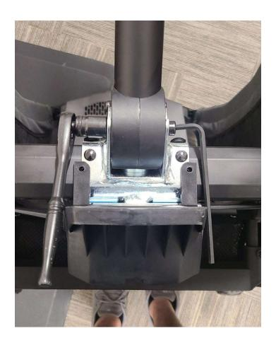
Step 6: Remove the lock pin. Verify you have all of the parts shown below.
