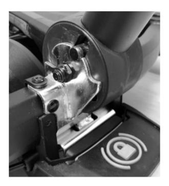
Step 5 : Remove handle pivot nut, washer and bolt using the wrench and hex wrench. Lift handle out of Cruiser.
