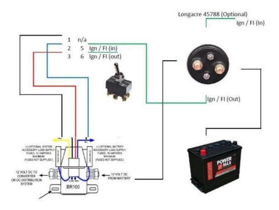
Diagram shows how to connect this system into any race car.
