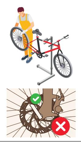
Warning: Improperly adjusted and closed wheel quick-release mechanisms may become active and get caught in the spokes or brake discs. This can lead to the wheel loosening or accidentally detaching, creating an additional risk of loss of control, falling, and even severe injury or death. Before each ride, be sure to properly adjust and close the quick-release mechanism.
