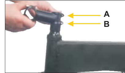
03 Tighten the side A, B screws
