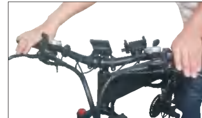
06 Adjust handlebar according to your needs , then ensure all bolts are tightened firmly
