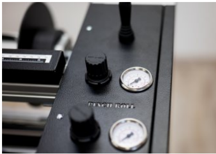
Adjustable pressure for pinch rolls and vertical blade
