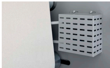
Felt belt automatic tracking system by PLC
