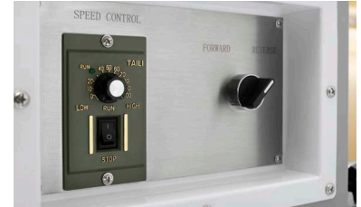
Rear rewinding shafts speed control
