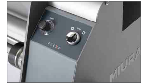
Speed regulator and switch to adjust the rotation of the rewinding shafts
