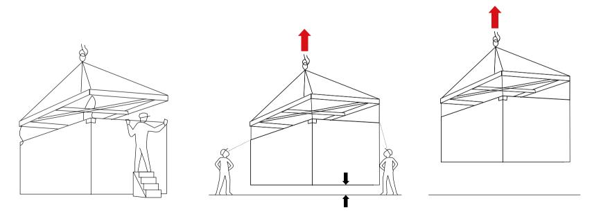
Having performed these checks, proceed with the lifting and handling of the container, with smooth controlled movements, avoiding tilting. Choose a location in accordance with Section Unloading and handling. General instructions. Once it is placed on the ground, after checking the correct stability of the container, the slings may be loosened and removed.
