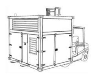
According to the weight of the genset, the machinery used must be checked to ensure it is able to carry the load in a safe and controlled manner.
