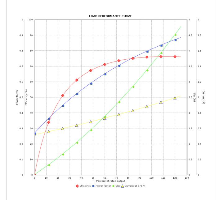
Performance : 575 V 60 Hz 2P Rated current : 0.920 A Moment of inertia (J) : 0.0356 sq.ft.lb **LRC** : 7.7 Duty cycle : Cont.(S1) : 1.13 ft.lb Insulation class : F Rated torque Locked rotor torque : 380 % Service factor : 1.15 Breakdown torque : 400 % Temperature rise : 80 K Rated speed : 3470 rpm
