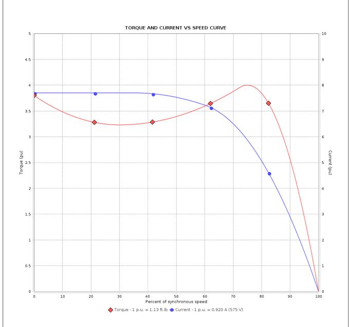
Performance : 575 V 60 Hz 2P Rated current : 0.920 A Moment of inertia (J) : 0.0356 sq.ft.lb **LRC** : 7.7 Duty cycle : Cont.(S1) : F Rated torque Insulation class : 1.13 ft.lb : 380 % Service factor Locked rotor torque : 1.15 Breakdown torque : 400 % Temperature rise : 80 K Rated speed : 3470 rpm
