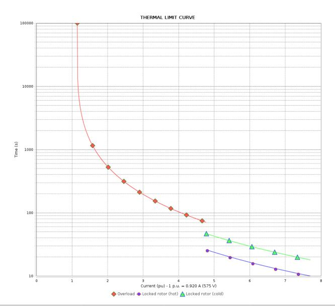
Performance : 575 V 60 Hz 2P Rated current : 0.920 A Moment of inertia (J) : 0.0356 sq.ft.lb **LRC** : 7.7 Duty cycle : Cont.(S1) : 1.13 ft.lb Insulation class Rated torque : F Locked rotor torque : 380 % Service factor : 1.15 : 400 % Breakdown torque Temperature rise : 80 K Rated speed : 3470 rpm Heating constant
