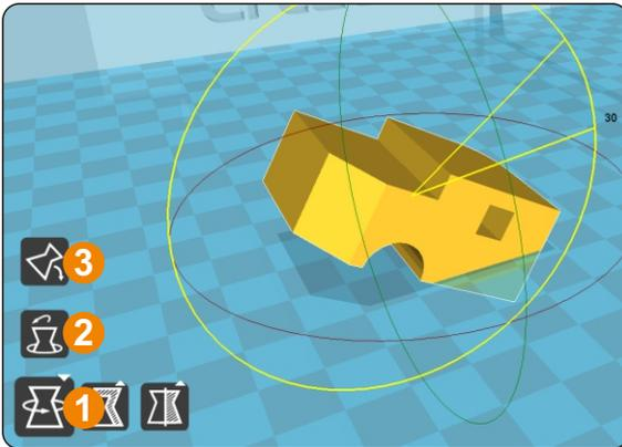
Click on the left corner of the rotate button [1], you can see three ring line around the model, respectively along the X, Y, Z direction. The default rotation angle is 5 degrees, press the Shift key can restrict the rotation angle to 1 degree.
