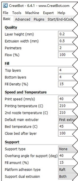
**Layer height:** This is the most important setting to determine the quality of your print, maximum value not exceed 80% of the nozzle diameter.
