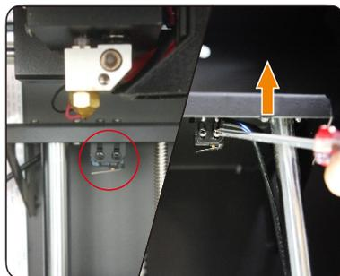
If the nozzle can't touch the platform even loosen all the leveling nut, you can move Z stop limit a little up, as you can see from figure.
