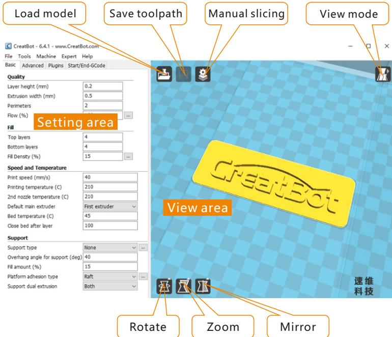
As you can see from the complete UI, the left side of the software is setting area, the right side is view area. The setting area contain "Basic", "Advanced", "Plugins", "Start/End GCode" four tabs. The Basic tab is the most common settings, usually the most frequently used parameters are here. Each parameter has a mouse-over tips, you can set parameters according to the prompt. If you want to restore the default settings, please click on the menu "Tools"->"Restore Default".
