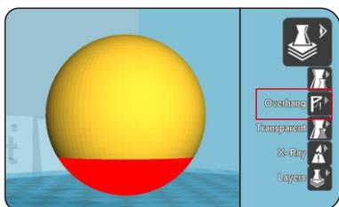
From the overhang view, you can see the suspended part of the model which is shown in red color. By changing the supporting angle can be seen suspended parts size is dynamically changing.
