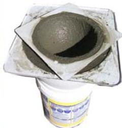
**Option:** If you are casting two sizes of half balls you may take advantage of casting the second half inside the bigger one. This will make the ball hollow, save material and make the ball lighter weight.
