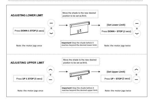
**Tips:** If you hold the UP/DOWN button for more than 3 seconds, the shade will enter running mode. As the shade approaches the desired limit, press the STOP button and then fine-tune the limit.
