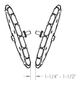
SPACE WHEELS AT APPROXIMATELY 1-1/4", GAP MAY NEED TO BE ADJUSTED BASED ON PLANTING CONDITIONS. THE NUMBER OF SPACERS USED WILL VARY DEPENDING ON THE PLANTERS TAIL UNIT. IN SOME CASES, ADDITIONAL SPACERS MAY BE NEEDED OR NOT ALL OF THE PROVIDED WASHERS WILL BE USED. PLANTING CONDITIONS VARY, SO IT WILL BE NECESSARY TO CHECK FOR SEED TO SOIL CONTACT & THE CONDITION OF THE SEED FURROW.
