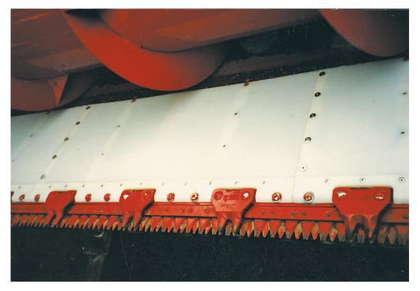
Step 6. Install the remaining panels working from the center towards each end. Make sure the metal clips on the bottom side of the poly panels are inserted into the slots that they originally were in on the header.
