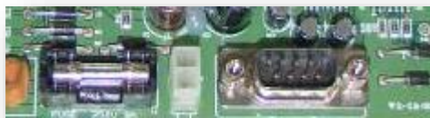
24VDC Power Input Bill Dispenser Communication
