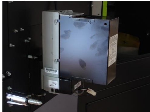
Figure 6 – Bill Stacker Attached to Bill Acceptor
