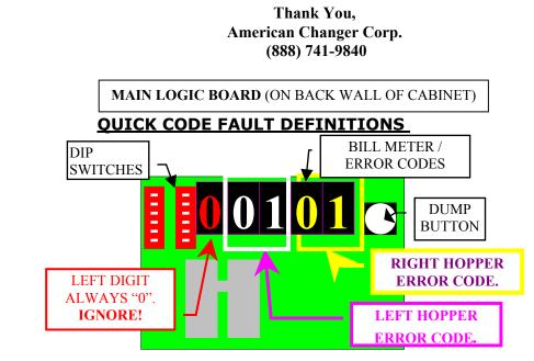
Press the "DUMP" Button before turning off changer. Match the code to samples below to find out why the hopper(s) were shut down
