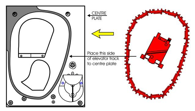
2. Once the 'track plate' is in position, turn the track through  $720^{0}$  to ensure it is seated in the guide path correctly.
