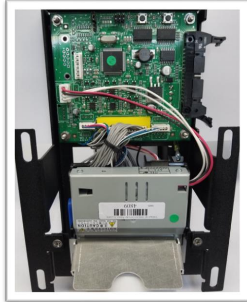
Printer Out Jumper Placement
