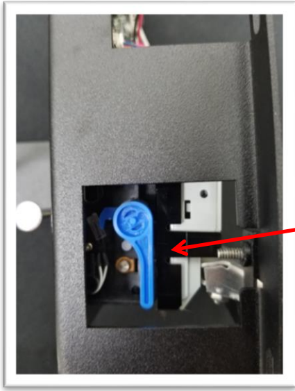
Paper Feed Lever in the down position
