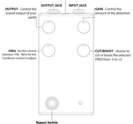
Press to activate/deactivate the pedal. The pedal will remember the state it was last in and boot up in that state.
