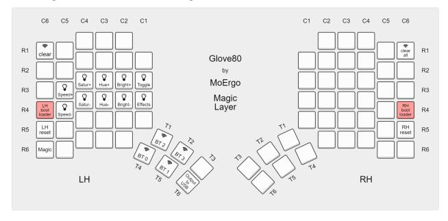
The simplest way is to use the key mapping on the ZMK key layout by activating the &bootloader behavior on the half of the Glove80 that you want to load new firmware. On the default key layout, you can do so by
