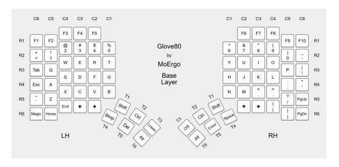
Please note that legends in the illustration above, R1...R6, C1...C6, and T1...T6, define the convention for key positions on Glove80. For example, in the default layout Base Layer, LH C2R3 is "R", and RH T1 is the "Shift" key on the right hand.
