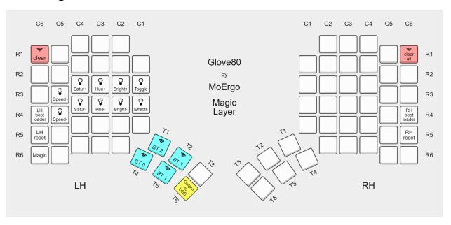
On a default key layout, you can select a BT Profile by pressing the Magic Key and the corresponding key highlighted in blue above.
