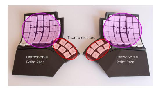
Contoured keywell: Keys to type with your four fingers on each hand
