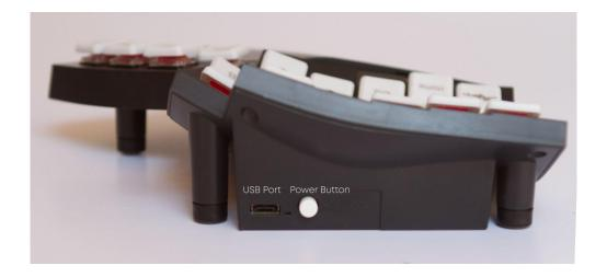
Power button: For switching off power. Please note that it is still possible to charge the battery even when powered off.
