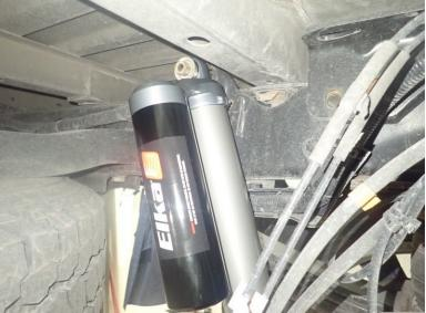
• ON REAR LEFT SIDE: install shock with reservoir facing Inside the vehicle as shown.
