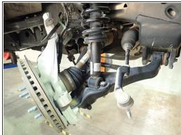
Remove upper arm ball joint nut and tie rod end ball joint nut, then separate them from steering knuckle.
