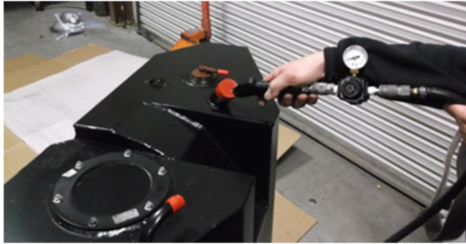
Figure 23: Pressure test the tank
