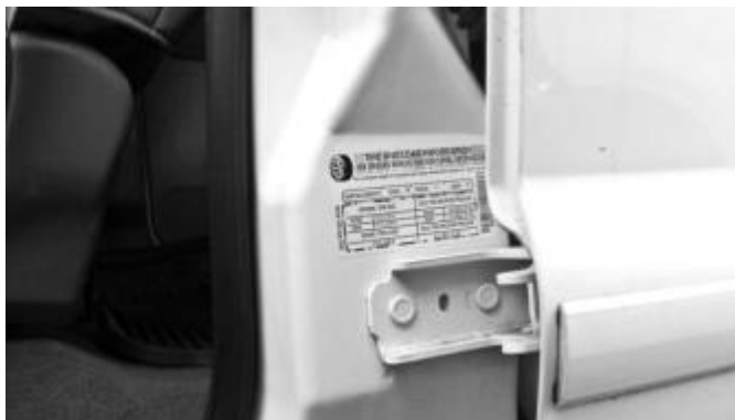
Figure 36: Affix Door Post and Tire and Loading Labels
