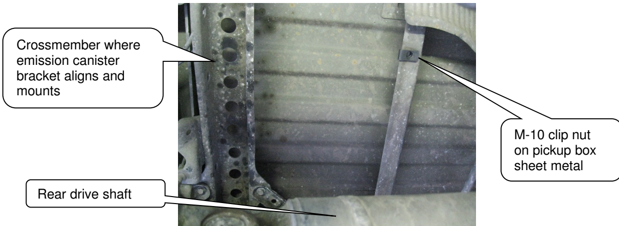
Figure 11: Install M-10 clip nut in sheet metal
