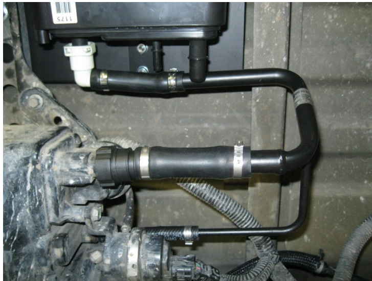
Figure 16: Installed emission tube assembly
