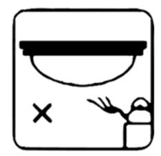
DO NOT install around high temperatures or humid environments
