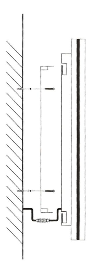
**NOTE:** After carrying out the load-bearing test of the luminaire, then after install the appropriate expansion screws according to the installation site environment.
