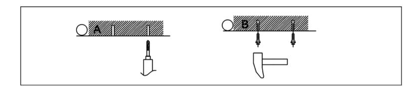
II. FIX THE HANGING BOARD TO THE WALL WITH SELF-TAPPING SCREWS AND CONNECT THE POWER CORD.
