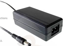
The Tiger Power range of switch mode power supplies feature full safety approvals and meet latest level VI energy efficiency requirements. The TP1132 24vdc 1.25 amp model provides a reliable constant voltage output at up to 30 watts continuous, suitable for a wide range of applications.
