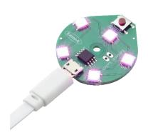
The board has 4 patterns, selected by pressing the button to step through them There is an additional off position after the 4<sup>th</sup> pattern:
