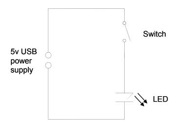
The circuit diagram for the USB lamp is shown above. It is a very simple circuit. The 5V that powers the circuit is supplied from the USB connector.
