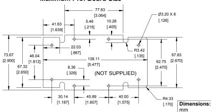
Enclosures can be Factory Modified (Milling, Drilling, Printing etc.) Contact Factory mjm@hammondmfg.com for quotes Solid models of this enclosure available in STEP or IGES. (Part number and text placement/orientation on our products are subject to change,
