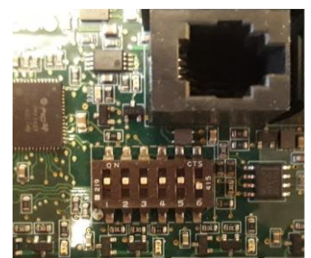
Figure 6 DIP switch positions for using a heater
