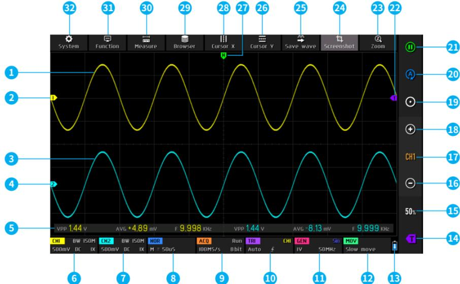
①The signal waveform of channel 1 is displayed in yellow brightness when the color temperature is turned off. The brighter the area, the greater the probability of the area appearing. When the color temperature is turned on, it is displayed as a color transition. The temperature gradually increases from blue to red, which means the probability of the area appearing is greater.
