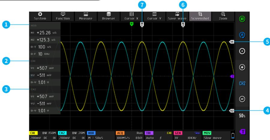
①Parameter bar of time cursor X, where H1/H2 refers to the time of H1/H2 cursor line relative to the coordinate center. D-T refers to the absolute value of the time difference between H1 and H2. D-F refers to the frequency value corresponding to the H1 and H2 cycles.
