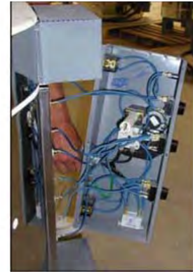
Remove wires from back of kiln sitter terminal block.
