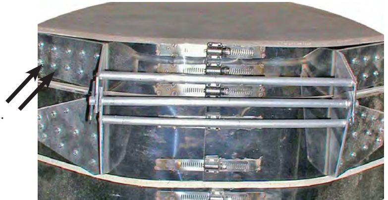
Repositioning Lid when Thermal Expansion Occurs
