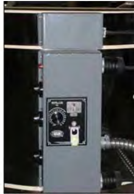
Detach screws from kiln sitter plate.
