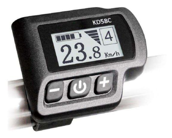
The LCD display unit will come pre-mounted to the handlebars of the Tower Beach Bum and Beach Babe. This section covers the general operation of the LCD display unit. A more comprehensive manual for the unit is included in the eBike packaging, and on towerelectricbikes.com.
