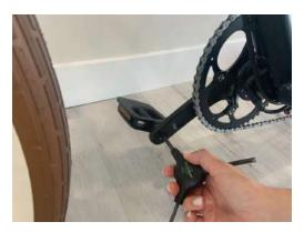
Begin the installation by twisting the pedal into the correct pedal arm by hand. Once the pedal becomes too difficult to twist by hand, further tighten with an M6 hex wrench.
