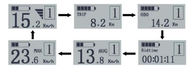
Each interface will display for 2 seconds before automatically returning to the Running Speed interface.
