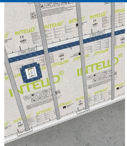
Use LESSCO Box to create an airtight cavity for light switches and electrical outlets when there is no service cavity. Tape LESSCO Box to the membrane with TESCON VANA.
