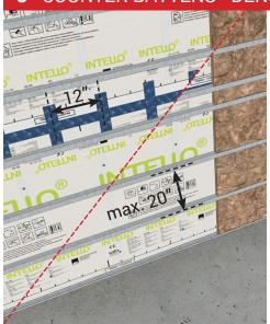
Add horizontal counter battens spaced max. 20" apart before dense packed insulation is blown in. Tape joints should be supported with a batten over the tape or reinforced with perpendicular strips of tape spaced less than 12" apart.
