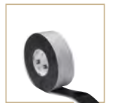
TESCON Naidec Double sided butyl tape to seal screw and nail penetrations under battens. Recommended on low pitched roofs and severely exposed walls (open joints, coastal, high wind areas)
