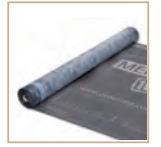
SOLITEX MENTO 1000 Weather resistive barrier /roof-underlayment made from monolithic TEEE-membrane and PP protective layers. UV-resistant. Up to 3 months of weather exposure.
