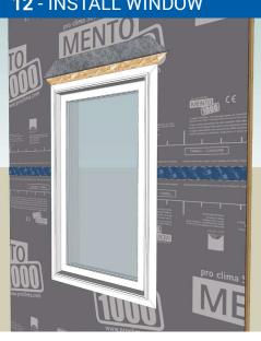
Install the flanged window and fasten to structure per manufacturer's instructions.
