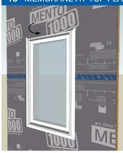
Unfold the membrane and run it over the top flange.
