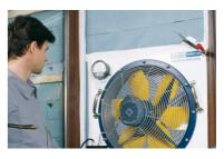
When all connections have been made air-tight, the thermal insulation system is secure for the longterm. It is recommended to check the air-tightness using a BLOWER DOOR or a pro clima WINCON.
