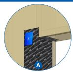
A - Cut the required length of tape (jamb height + 4" (100 mm)). Apply narrow and middle strips of tape to sheathing, centering the tape on the edge of the window side. Start 1" (25 mm) below the lower sill. Align edge of the release paper with the rough opening. The tape should end approx 3" (75 mm) above the window head. Cut the third release strip using a utility knife along the window head edge. Fold the tape into the opening and adhere to R.O. Press accurately into the corner with PRESSFIX.
