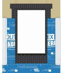
Apply ADHERO to sides of R.O. Overlap ADHERO at least 3" (75mm) over CONTEGA SOLIDO EXO on sides and a minimum of 4"-6" (100-150 mm) over ADHERO below. Pressurize using PRESSFIX XL.
