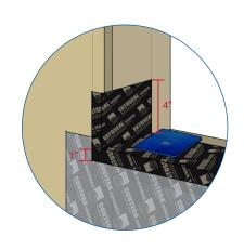
Install EXTOSEAL ENCORS on window sill, extending it up each side a minimum of 4" (100 mm). Use PRESSFIX to accurately press into corners
