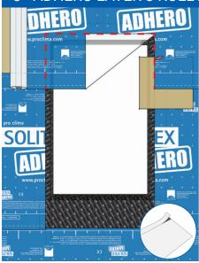
Apply ADHERO over the head of the window. Adhere top 10" (250 mm) wide strip first. This will allow you to trim excess material at window opening without damaging CONTEGA SOLIDO EXO tape below.
