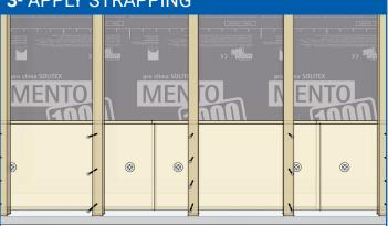
Mark the vertical centers for strapping. Use 1x4 or 2x lumber for strapping. Use a level to ensure even application. It is recommended to apply at least 7 fasteners per board through the strapping back to the structural stud. (See 'Fasteners' section at the end of this page).
