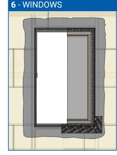
Cut boards to allow for the opening of the window. Stagger vertical joint from the line of the window buck by a minimum of 12" (300mm). Apply a minimum of 2 coats of VISCONN liquid applied membrane or 1 layer of TESCON PRIMER RP to window head, jamb and sill to act as priming layer. Apply EXTOSEAL ENCORS tape to flash the window sill and 4" (100 mm) up the jamb. Once the window has been installed the window should be taped using either TESCON VANA, CONTEGA SOLIDO EXO or a combination of both.
