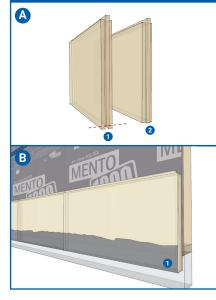
A - Cut off the bottom groove of the board (1) to create a level surface (2). Use a laser level, chalk, or pencil to mark a line on the substrate. The board must be installed at a minimum of 6" (150 mm) above grade.
