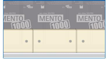
Apply the first group of boards making sure the board tongue and grooves are tightly fitted. Apply so that the GUTEX name and branding text is facing outwards. Secure boards in place with screws and insulation disks - install disks flush with face of board to avoid inteference with battens. Alternatively a 2x can be used as temp. starting ledge as well.
