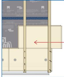
Slide the next set of boards behind the strapping, making sure the tongue and grooves are tightly fitted. Stagger the vertical joints from row-to-row by a minimum of 12" (300 mm).
